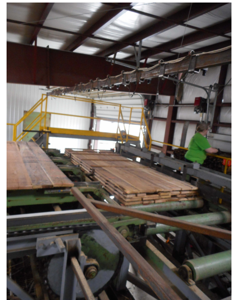
Stacking lumber for drying. It is essential to provide ventilation between the layers of boards. This is accomplished with stickers, which are laid in place using laser guidance.
