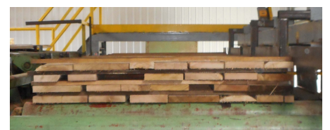
Stickers, which are narrow strips of wood used to separate layers of boards, allow for air flow during the drying process.
