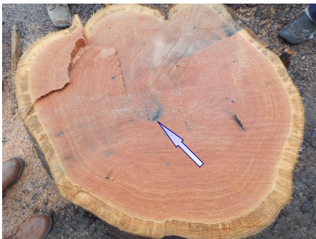
Metal detection in timbered logs is noted by the dark stain deep within the tree.
