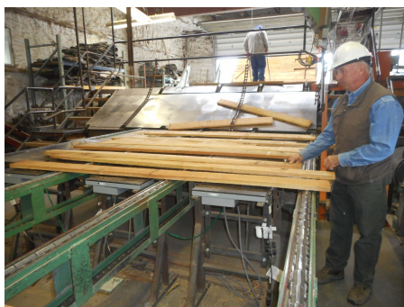
Capacitance meters along the line inspect every board for moisture content.
