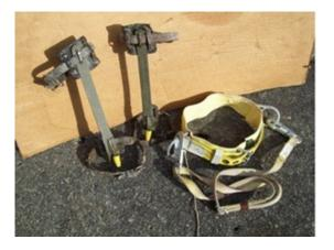
**For Sale:** Steel Tree/Pole Climbers, contoured and offset with snap-on Gaff Guards. Lightweight Nylon Body Belt with D-Rings and Pole Strap, OSHA Standards. See photo below. \$200 for both. Contact Dale at 585-367-2849.
