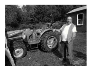
Charles cuts and moves firewood and sawlogs with the help of a Massey Ferguson model 1540, 40 h p, 4-wheel drive, and a 4 1/2 ton winch. The loader will
