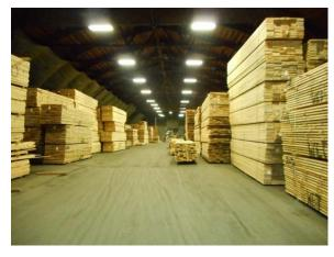
After the lumber is graded, it is stacked in the warehouse for natural air drying. No heat is used in drying the lumber.
